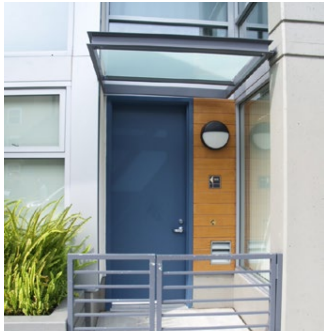
Private residential street-level entrances shall be set back to provide space for front porches or small entry courts.
