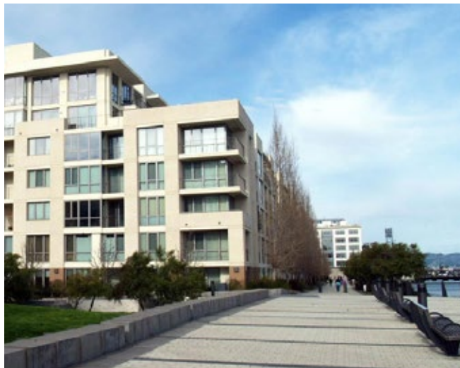
Stepbacks make building heights less imposing and create variation in building massing.
