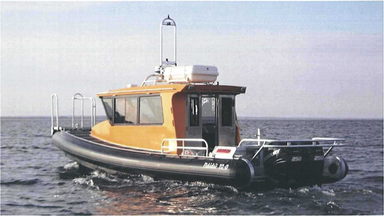
PD Industries – 10 meter cabin boat with D-shaped foam core fender system
